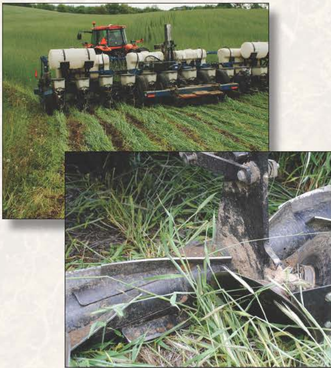
Figure 20. A cover crop roller/row cleaner system designed by a Pennsylvania farmer/engineer from Perry County. It can be attached to a corn planter. It parts the cover crop in front of the double disk. (Courtesy of Sjoerd Duiker)
