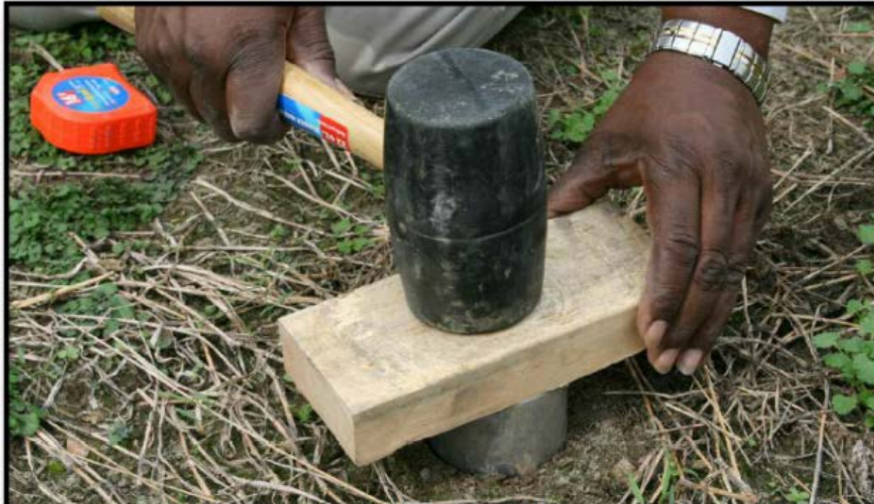
A three inch diameter ring is hammered into the soil to collect bulk density samples. Ref.: NRCS Soil Quality Indicators
