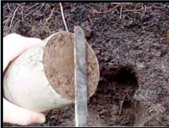
A three inch diameter ring is hammered into the soil to collect bulk density samples. Ref.: NRCS Soil Quality Indicators
