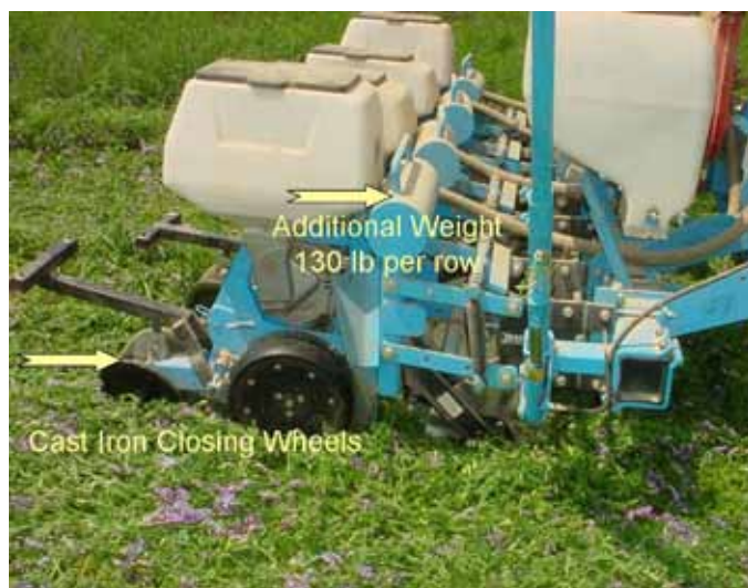
No-till Monosem planter with modifications
