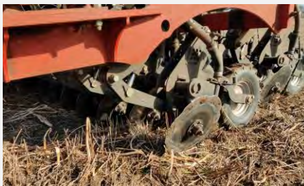
Example of a no-till disc seeder
