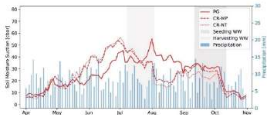
Fig. 4 Average SMS fluxes and precipitation sums for Oberacker in common years (WW= winter wheat).
