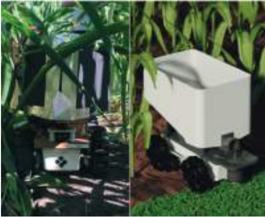
Fig #1: Earth Sense's autonomous robotic cover crop seeder, actual on left, model on right
