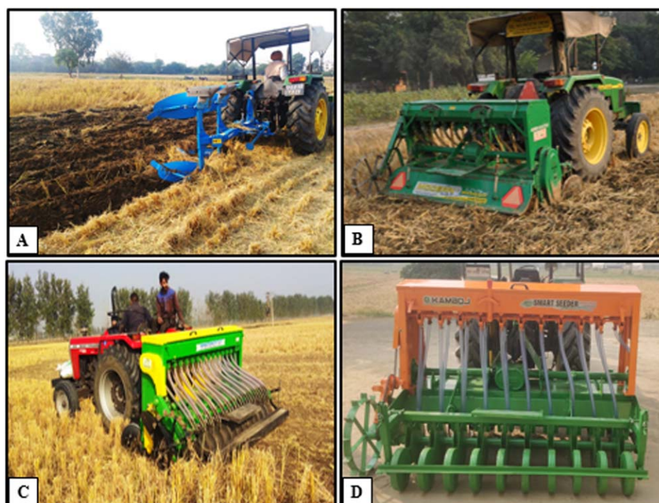
Figure 9. Different rice straw management machineries. (A). MB Plough, (B). Roto-till-drill, (C). Super seeder, (D). Smart seeder).
